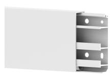
E skirting trunking made of PVC according to DIN EN 50085-2-1 for cable laying on the wall, consisting of a base with grooved back for fixing with mounting adhesive and three separate chambers for cable laying/separation as well as a completely overlapping cover for snapping onto the base. The distance from the floor to the first occupancy chamber is 11 mm and thus fulfils the minimum distance to the floor according to DIN EN 50085-2-1.
